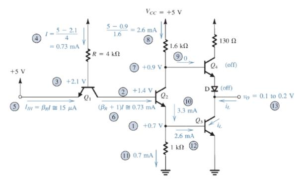
FIGURE x8.14 Analysis of the TTL gate with the input high. The circled numbers indicate the order of the analysis steps.
