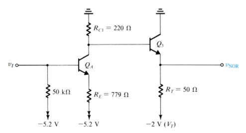
**Figure x8.29** Circuit for finding  $v_{\text{NOR}}$  versus  $v_I$  for the range  $V_I > V_{IH}$ .
