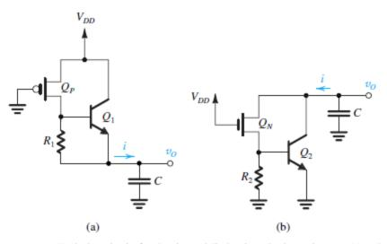
Figure x8.35 Equivalent circuits for charging and discharging a load capacitance C. Note that C includes all the capacitances present at the output node.
