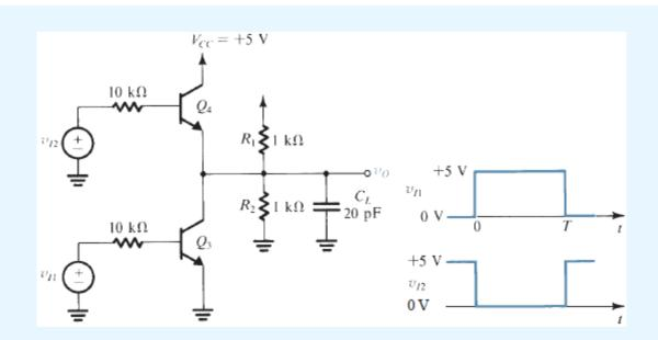
FIGURE x8.8 Circuit and input waveforms for Example x8.1.
