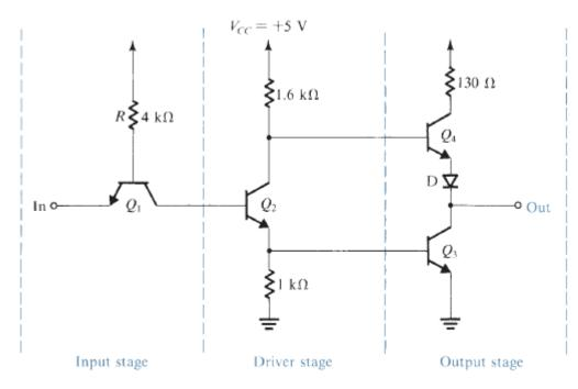
FIGURE x8.13 The complete TTL gate circuit with only one input terminal indicated.
