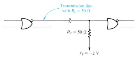
Figure x8.24 The proper way to connect high-speed logic gates such as ECL. Properly terminating the transmission line connecting the two gates eliminates the "ringing" that would otherwise corrupt the logic signals.
