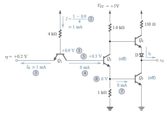
FIGURE x8.16 Analysis of the TTL gate when the input is low. The circled numbers indicate the order of the analysis steps.
