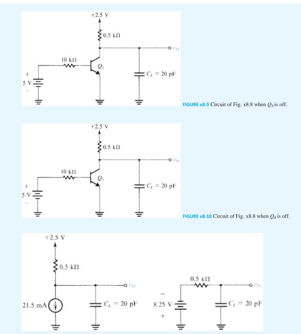
**FIGURE x8.11** (a) Equivalent circuit for the circuit in Fig. x8.10 when  $Q_3$  is in the active mode. (b) Simpler version of the circuit in (a) obtained using Thévenin's theorem.
