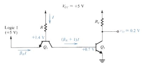
FIGURE x8.4 Analysis of the conceptual TTL gate when the input is high.
