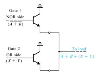
Figure x8.33 The wired-OR capability of ECL.
