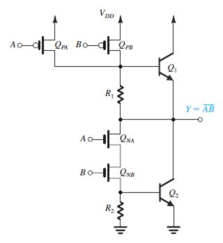
Figure x8.36 A BiCMOS two-input NAND gate.
