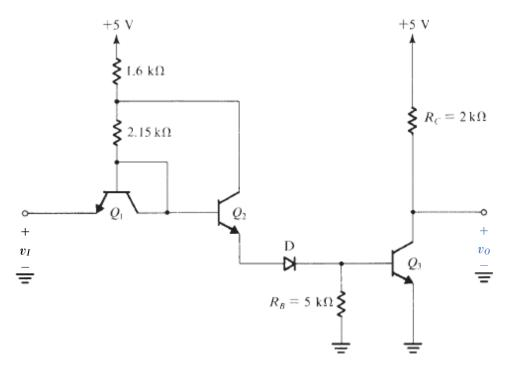
**FIGURE x8.1** IC form of the DTL gate with the input diode shown as a diode-connected transistor  $(Q_1)$ . Only one input terminal is shown.
