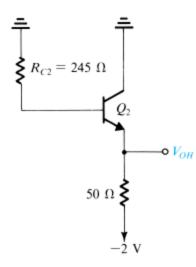
Figure x8.27 Circuit for determining V<sub>OH</sub>.
