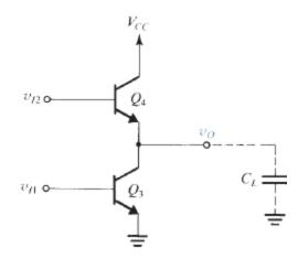
FIGURE x8.7 The totem-pole output stage.
