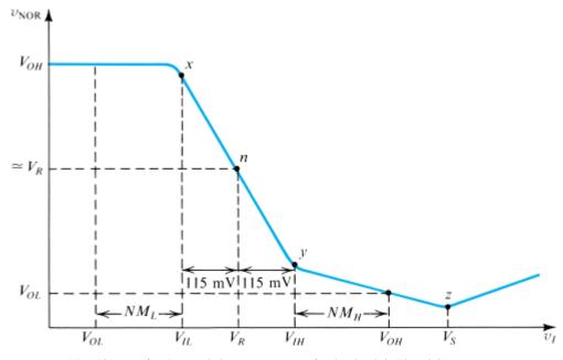
Figure x8.28 The NOR transfer characteristic,  $v_{NOR}$  versus  $v_I$ , for the circuit in Fig. x8.25.
