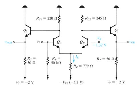
Figure x8.25 Simplified version of the ECL gate for the purpose of finding transfer characteristics.
