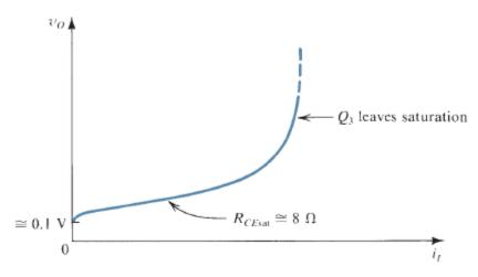
**FIGURE x8.15** The  $v_O$ - $i_L$  characteristic of the TTL gate when the output is low.
