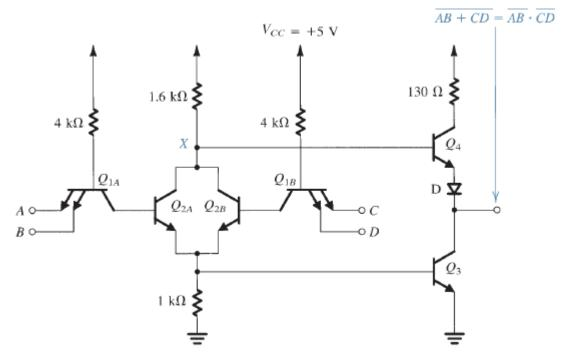
FIGURE x8.20 A TTL AND-OR-INVERT gate.
