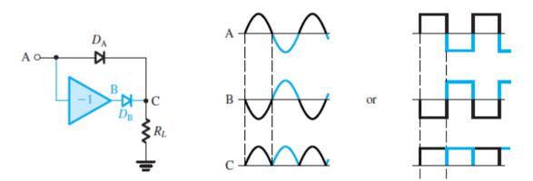
Figure x7.11 Principle of full-wave rectification.
