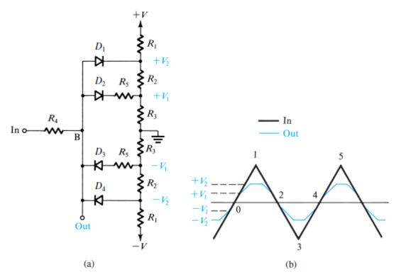
Figure x7.6 (a) A three-segment sine-wave shaper. (b) The input triangular waveform and the output approximately sinusoidal waveform.
