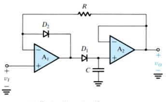
Figure x7.15 A buffered precision peak rectifier.
