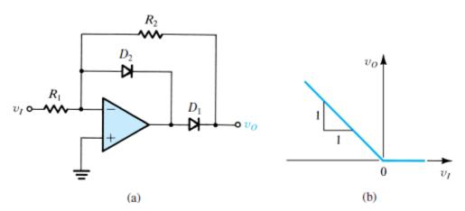
Figure x7.9 (a) An improved version of the precision half-wave rectifier: Diode  $D_2$  is included to keep the feedback loop closed around the op amp during the off times of the rectifier diode  $D_1$ , thus preventing the op amp from saturating. (b) The transfer characteristic for  $R_2 = R_1$ .
