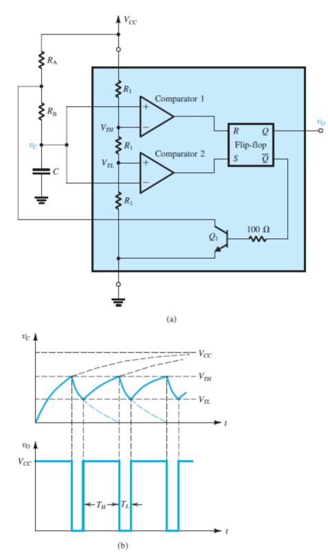
Figure x7.4 (a) The 555 timer connected to implement an astable multivibrator. (b) Waveforms of the circuit in (a).
