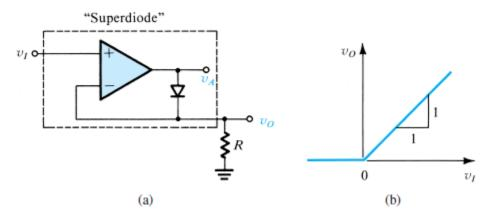
Figure x7.8 (a) The "superdiode" precision half-wave rectifier; (b) its almost ideal transfer characteristic. Note that when  $v_I > 0$  and the diode conducts, the op amp supplies the load current, and the source is conveniently buffered, an added advantage.
