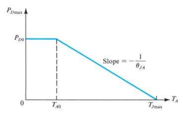
Figure x4.7 Maximum allowable power dissipation versus ambient temperature for a BJT operated in free air. This is known as a "power-derating" curve.
