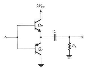
Figure x4.2 Class B output stage operated with a single power supply.
