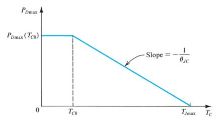
Figure x4.9 Maximum allowable power dissipation versus transistor-case temperature.
