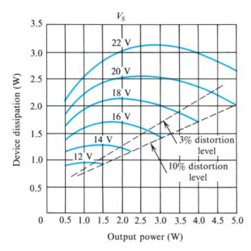
Figure x4.13 Power dissipation ( $P_D$ ) versus output power ( $P_L$ ) for the LM380 with  $R_L$  =8  $\Omega$ . (Courtesy National Semiconductor Corporation.)
