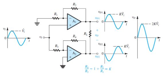
Figure x4.14 The bridge amplifier configuration.
