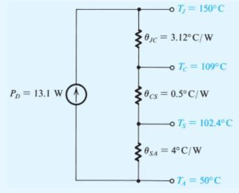
Figure x4.10 Thermal equivalent circuit for Example x4.2
