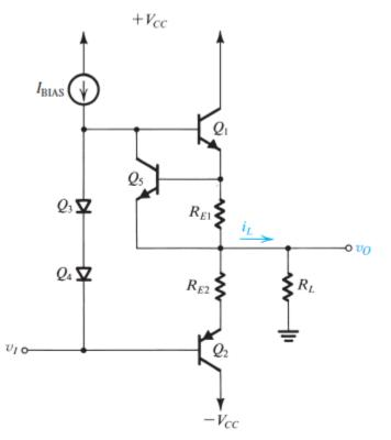
Figure x4.3 A class AB output stage with short-circuit protection. The protection circuit shown operates in the event of an output short circuit while  $v_0$  is positive.
