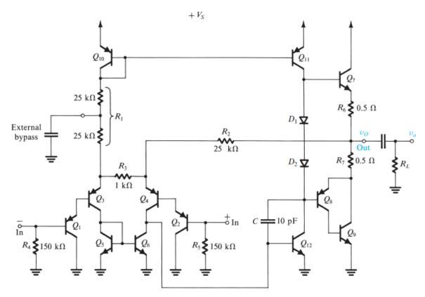
Figure x4.11 The simplified internal circuit of the LM380 IC power amplifier. (Courtesy National Semiconductor Corporation.)
