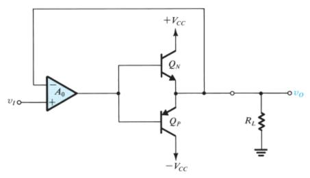
Figure x4.1 Class B circuit with an op amp connected in a negative-feedback loop to reduce crossover distortion.
