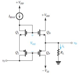
Figure x4.5 Classical CMOS class AB output stage. This circuit is the CMOS counterpart of the BJT circuit in Fig. 12.13 with the biasing diodes implemented with diode-connected MOSFETs  $Q_1$  and  $Q_2$
