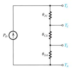
Figure x4.8 Electrical analog of the thermal-conduction process when a heat sink is utilized.
