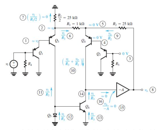
Figure x4.12 Small-signal analysis of the circuit in Fig. x4.11. The circled numbers indicate the order of the analysis steps.
