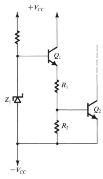
Figure x4.4 Thermal-shutdown circuit.
