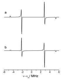
In the case of where A is described by [+5, +5, +10] MHz, the powder pattern resembles that shown in a) above. In the case of where A is described by [-5, -5, +10] MHz, the powder pattern resembles that shown in b) above. For the purely axial hyperfine shown in this example, the powder hyperfine pattern in b) resembles the Pake pattern shown for a purely dipolar system given in Fig. 5.14(c).
