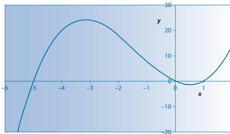
The highest power in the equation is 3 (there is an  $x^3$  term) so the maximum number of turning points in the graph is  $(3 - 1)$ , so 2.
