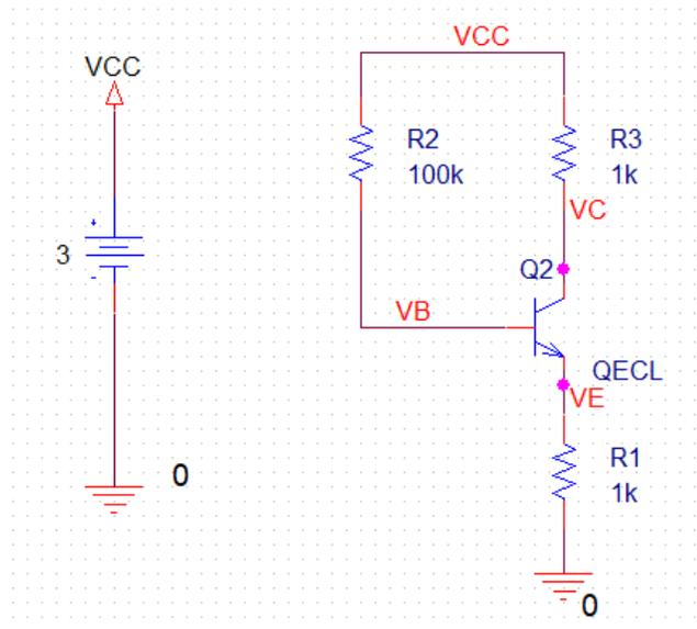
2. Run the netlist and calculate the operating point. Open the “output file” and see the node voltages and find out VB, VC and VE.
