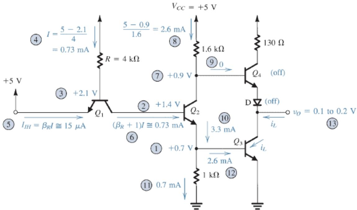
FIGURE x8.14 Analysis of the TTL gate with the input high. The circled numbers indicate the order of the analysis steps.
