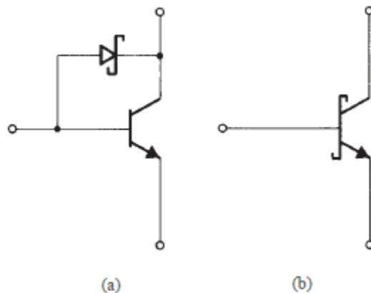
**FIGURE x8.21** (a) A transistor with a Schottky diode clamp. (b) Circuit symbol for the connection in (a), known as a Schottky transistor.
