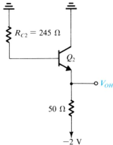
Figure x8.27 Circuit for determining  $V_{OH}$ .
