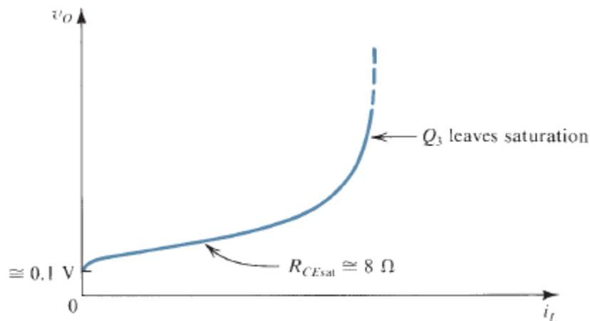
FIGURE x8.15 The  $v_O-i_L$  characteristic of the TTL gate when the output is low.
