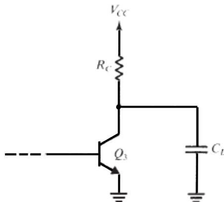
FIGURE x8.2 The output circuit of a DTL gate driving a capacitive load  $C_L$ .
