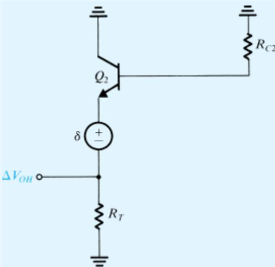
Figure x8.32 Equivalent circuit for determining the temperature coefficient of  $V_{OH}$ .
