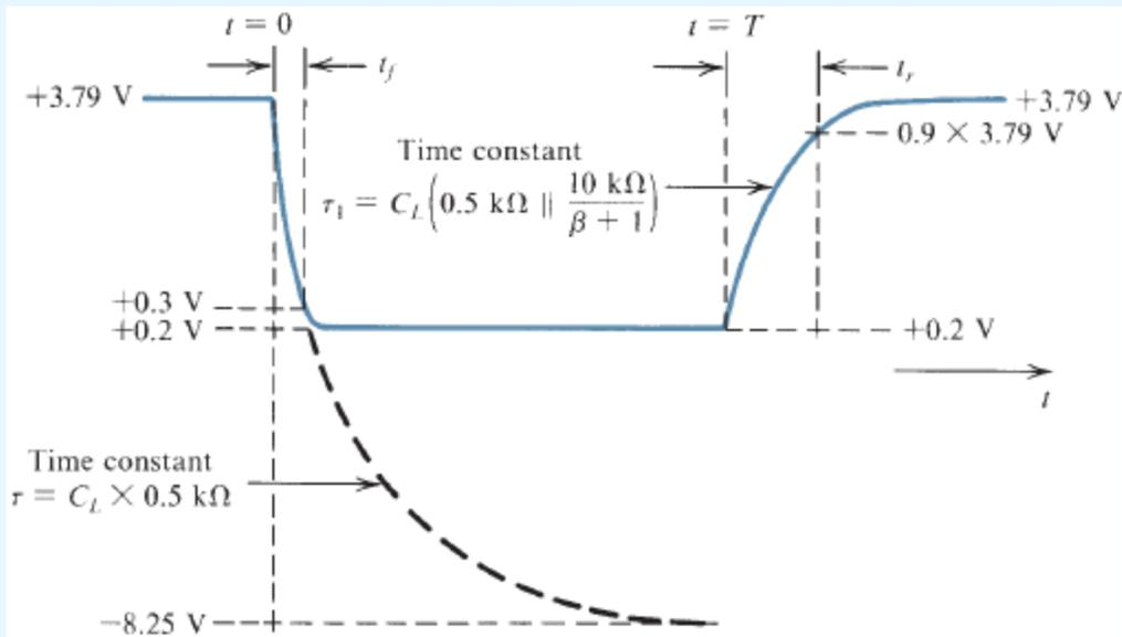
FIGURE x8.12 Details of the output voltage waveform for the circuit in Fig. x8.8.
