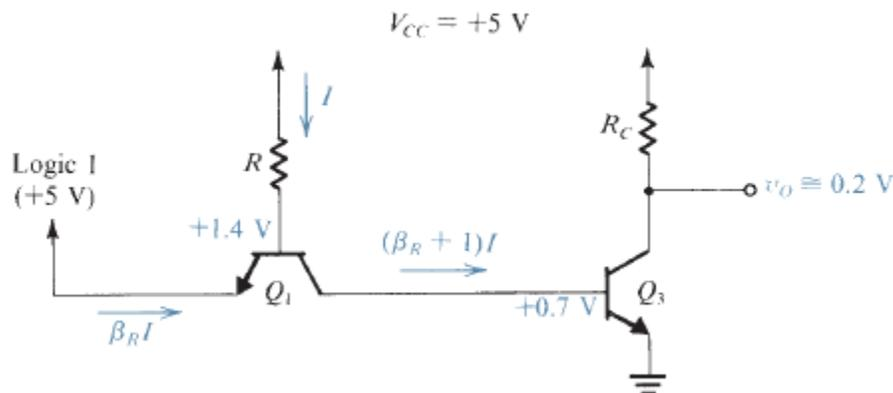
FIGURE x8.4 Analysis of the conceptual TTL gate when the input is high.
