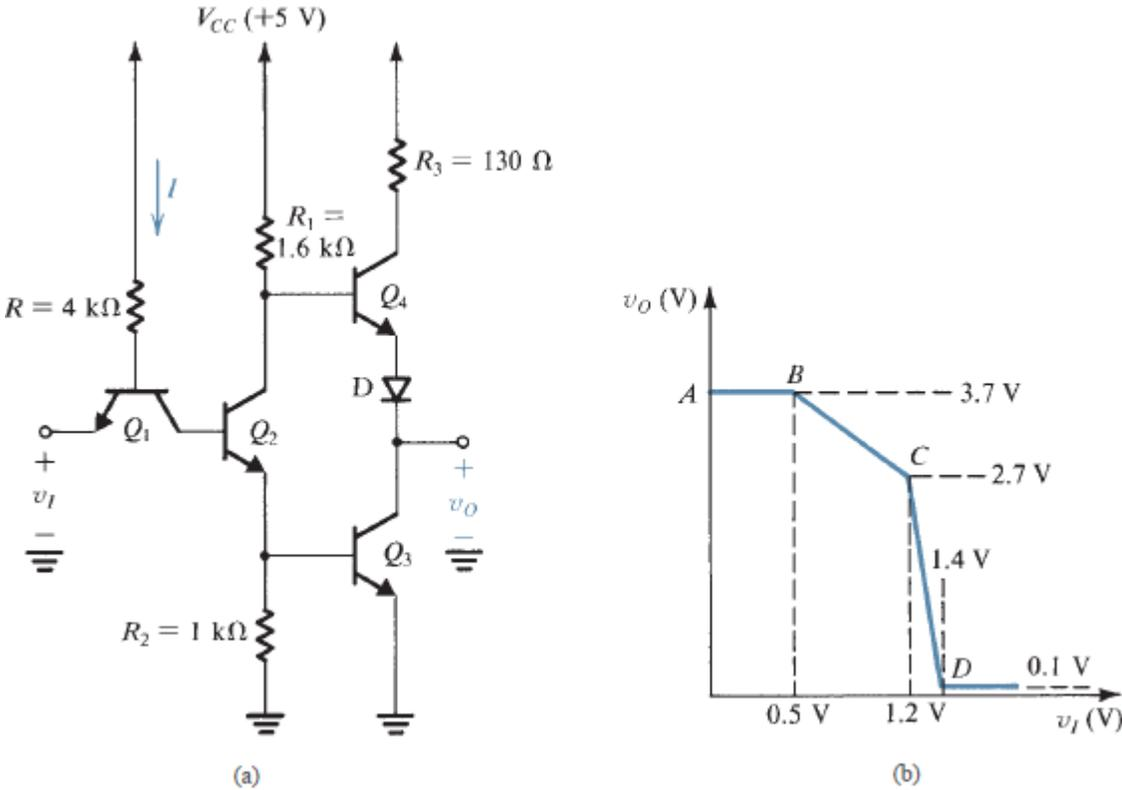
FIGURE x8.17 The TTL gate and its voltage transfer characteristic.
