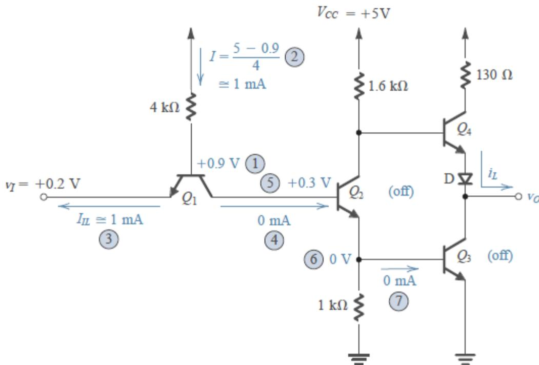
**FIGURE x8.16** Analysis of the TTL gate when the input is low. The circled numbers indicate the order of the analysis steps.
