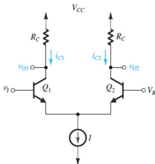
Figure x8.22 The basic element of ECL is the differential pair. Here,  $V_R$  is a reference voltage.
