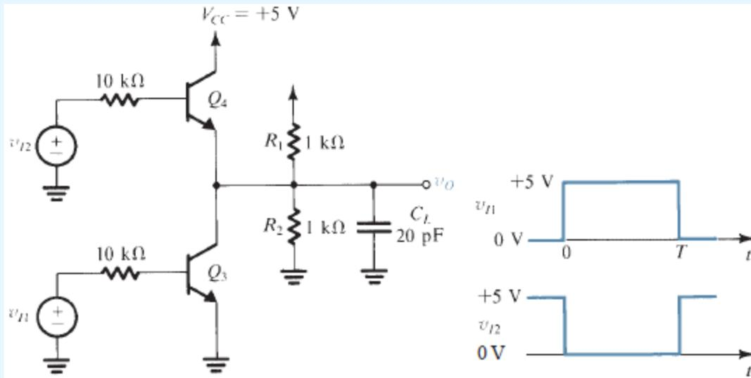
FIGURE x8.8 Circuit and input waveforms for Example x8.1.
