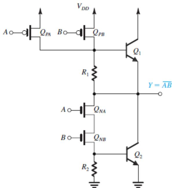
**Figure x8.36** A BiCMOS two-input NAND gate.
