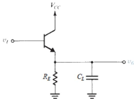
**FIGURE x8.6** An emitter-follower output stage with capacitive load.
