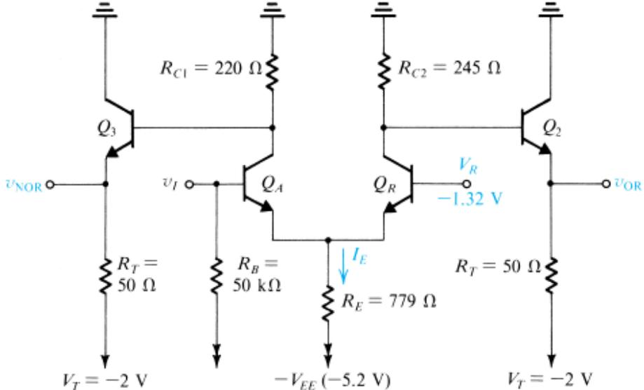
Figure x8.25 Simplified version of the ECL gate for the purpose of finding transfer characteristics.
