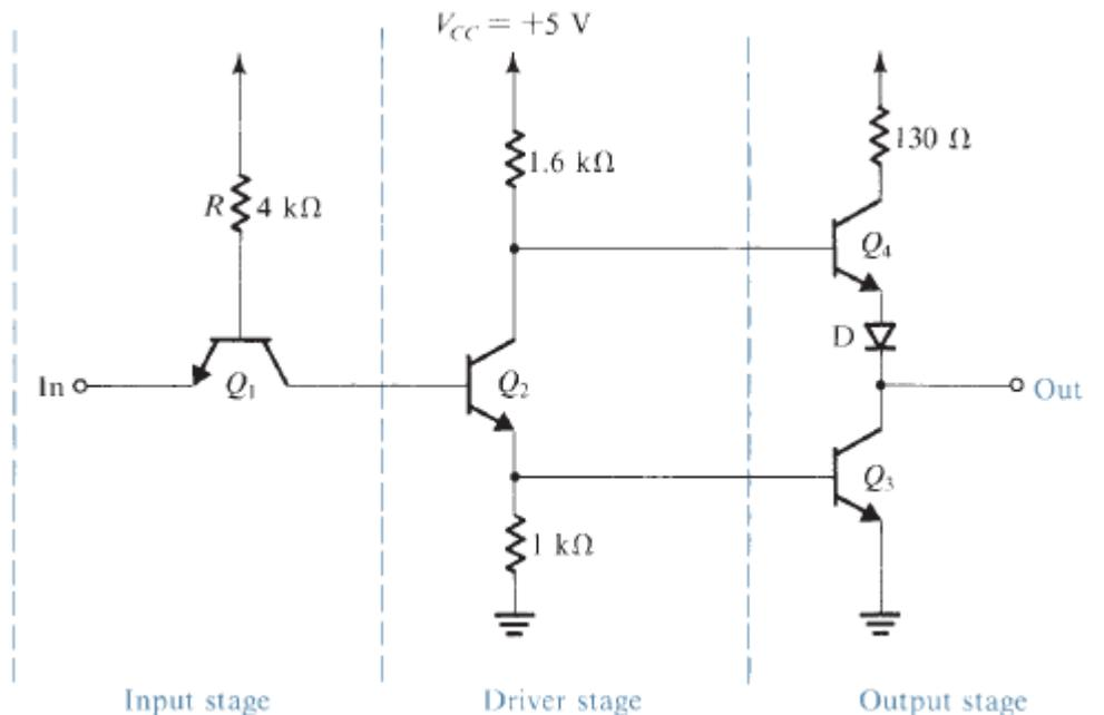
FIGURE x8.13 The complete TTL gate circuit with only one input terminal indicated.
