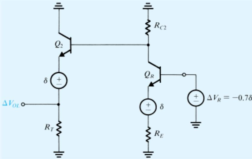
Figure x8.31 Equivalent circuit for determining the temperature coefficient of  $V_{OL}$ .
