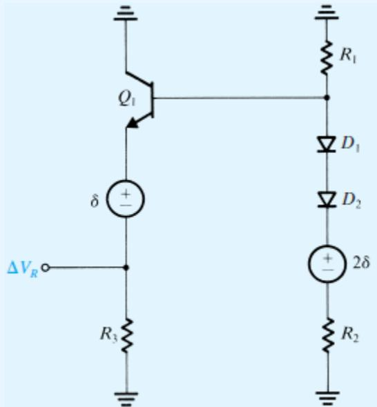
Figure x8.30 Equivalent circuit for determining the temperature coefficient of the reference voltage  $V_R$ .
