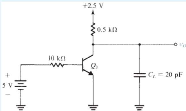
FIGURE x8.9 Circuit of Fig. x8.8 when  $Q_3$  is off.
