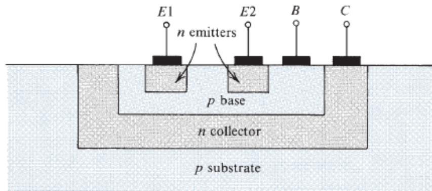
FIGURE x8.19 Structure of the multiemitter transistor  $Q_1$ .
