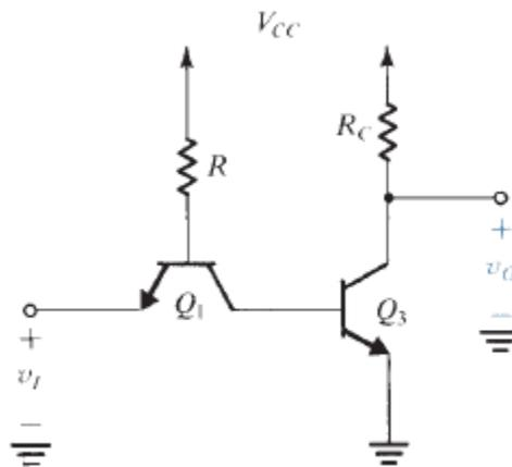
FIGURE x8.3 Conceptual form of TTL gate. Only one input terminal is shown.
