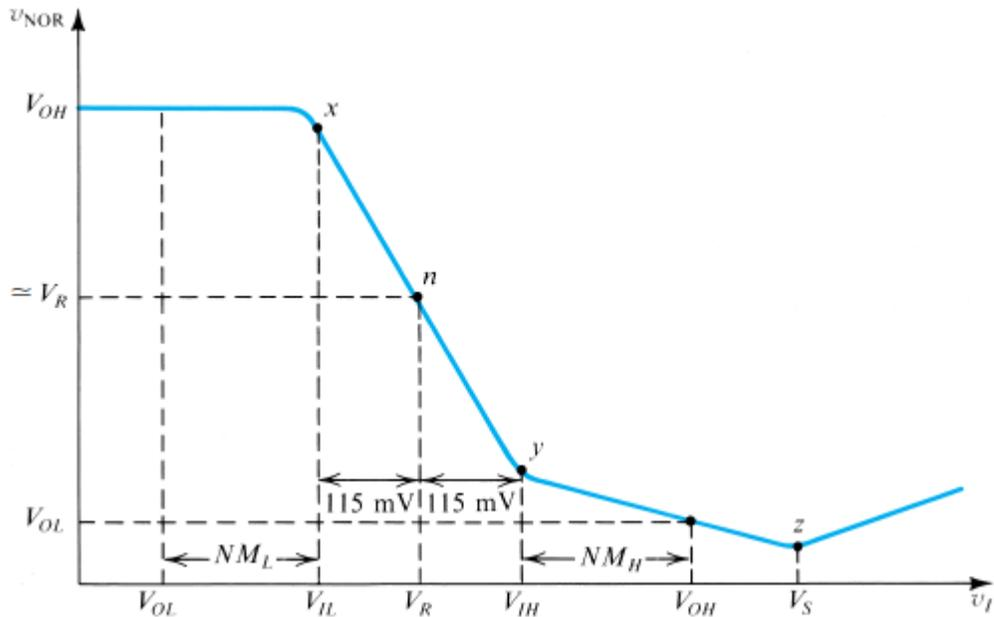
**Figure x8.28** The NOR transfer characteristic,  $v_{\text{NOR}}$  versus  $v_I$ , for the circuit in Fig. x8.25.
