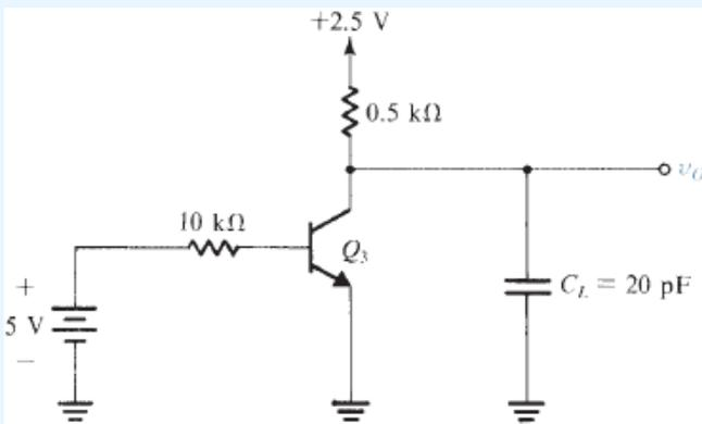
FIGURE x8.10 Circuit of Fig. x8.8 when  $Q_4$  is off.
