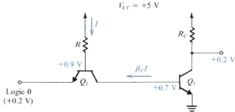
**FIGURE x8.5** Voltage and current values in the conceptual TTL circuit immediately after the input voltage is lowered.
