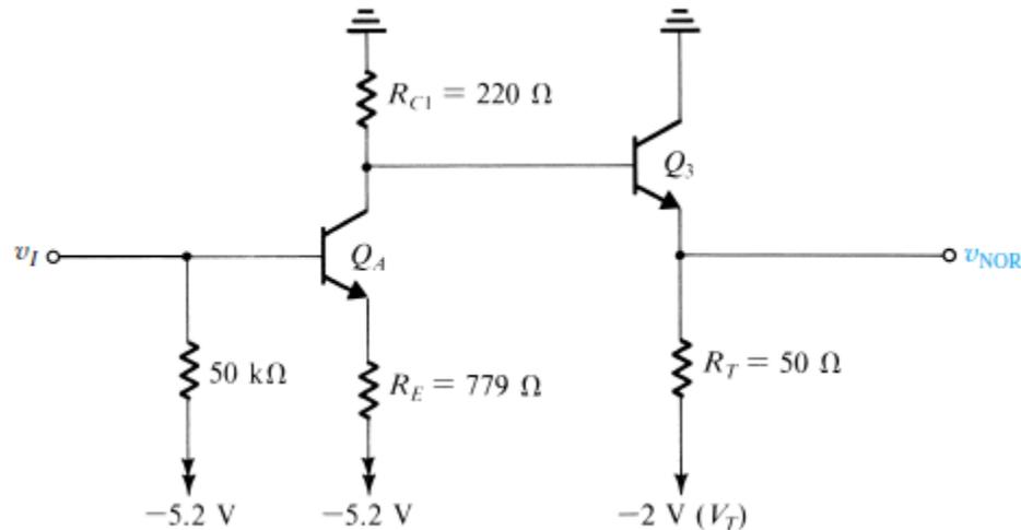
Figure x8.29 Circuit for finding  $v_{NOR}$  versus  $v_I$  for the range  $V_I > V_{IH}$ .
