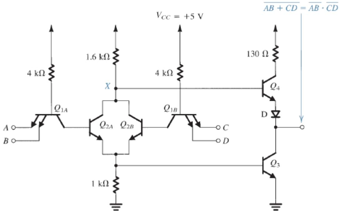
FIGURE x8.20 A TTL AND-OR-INVERT gate.
