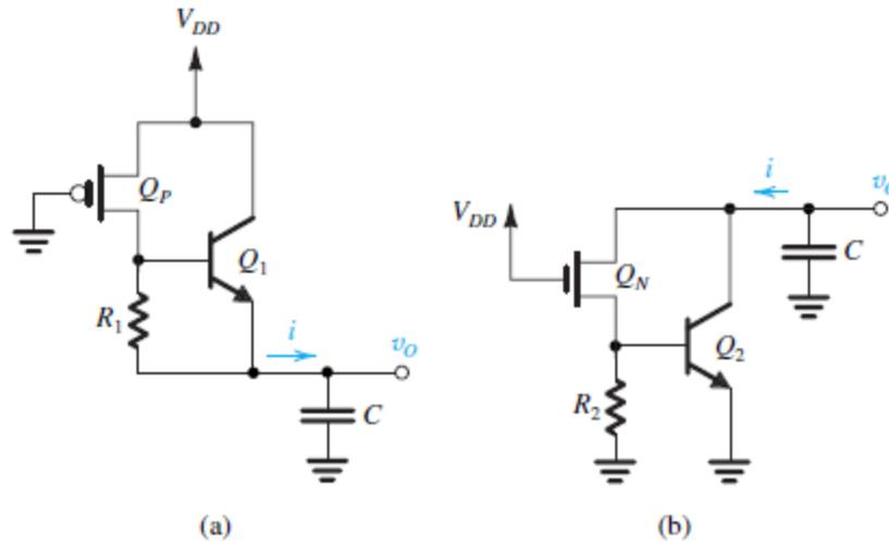
**Figure x8.35** Equivalent circuits for charging and discharging a load capacitance  $C$ . Note that  $C$  includes all the capacitances present at the output node.
