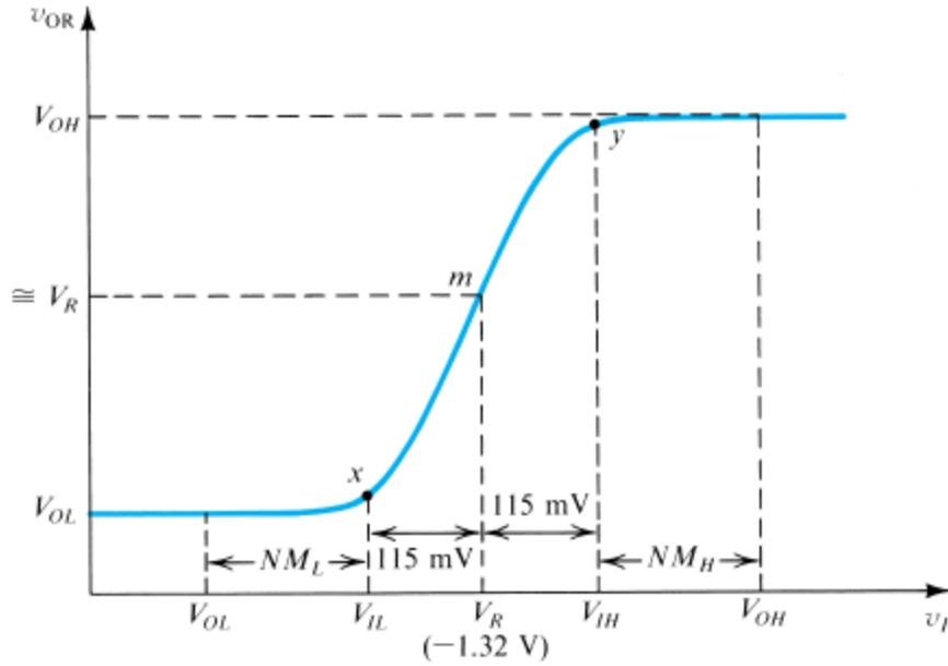
Figure x8.26 The OR transfer characteristic  $v_{OR}$  versus  $v_I$ , for the circuit in Fig. x8.25.
