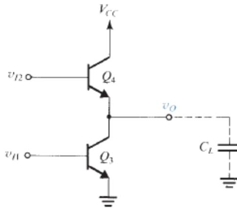
FIGURE x8.7 The totem-pole output stage.
