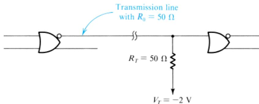
**Figure x8.24** The proper way to connect high-speed logic gates such as ECL. Properly terminating the transmission line connecting the two gates eliminates the “ringing” that would otherwise corrupt the logic signals.
