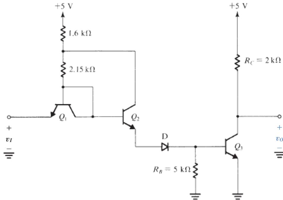
**FIGURE x8.1** IC form of the DTL gate with the input diode shown as a diode-connected transistor ( $Q_1$ ). Only one input terminal is shown.
