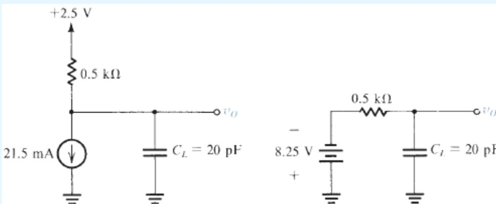
FIGURE x8.11 (a) Equivalent circuit for the circuit in Fig. x8.10 when  $Q_3$  is in the active mode. (b) Simpler version of the circuit in (a) obtained using Thévenin's theorem.
