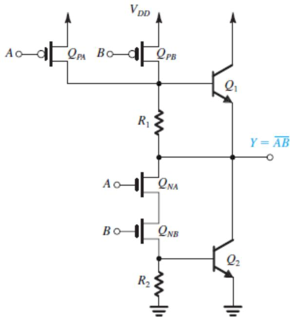
**Figure x8.36** A BiCMOS two-input NAND gate.
