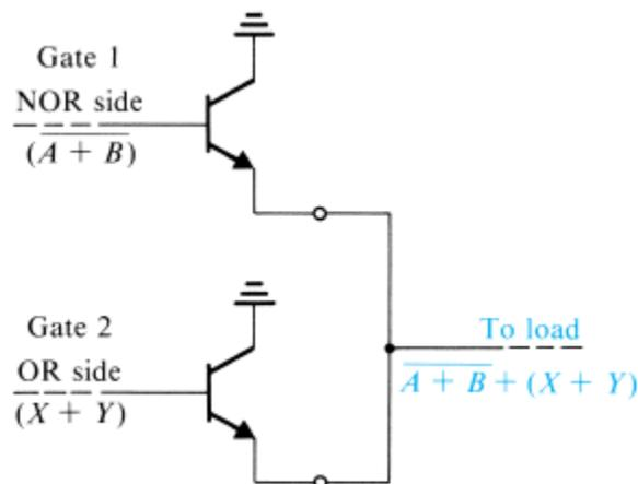
Figure x8.33 The wired-OR capability of ECL.
