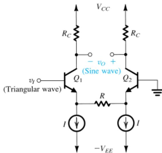
**Figure x7.7** A differential pair with an emitter-degeneration resistance used to implement a triangular-wave to sine-wave converter. Operation of the circuit can be graphically described by Fig. x7.5.
