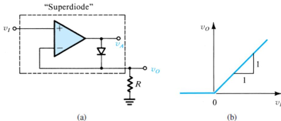
**Figure x7.8** (a) The “superdiode” precision half-wave rectifier; (b) its almost ideal transfer characteristic. Note that when  $v_I > 0$  and the diode conducts, the op amp supplies the load current, and the source is conveniently buffered, an added advantage.
