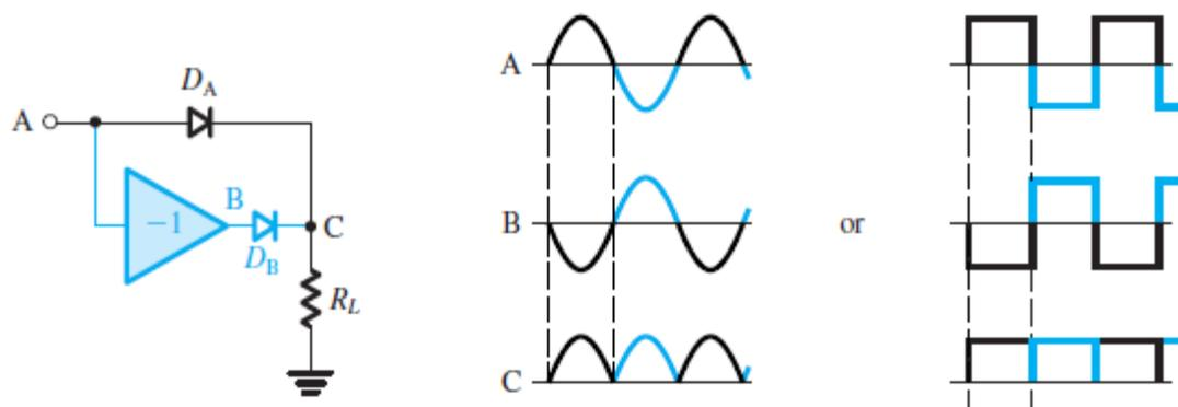
Figure x7.11 Principle of full-wave rectification.
