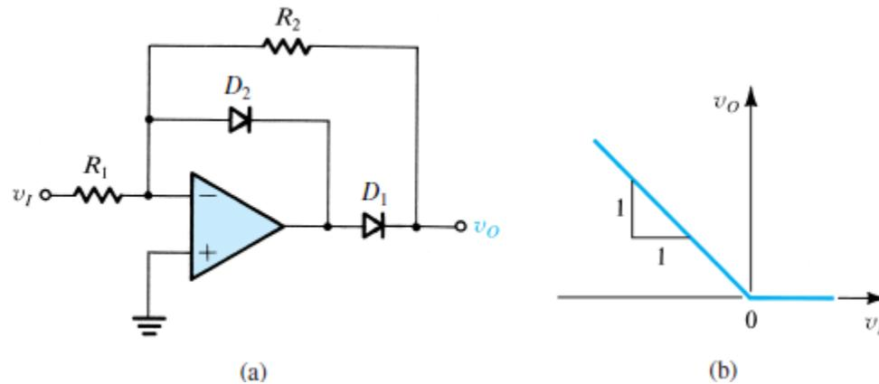
**Figure x7.9** (a) An improved version of the precision half-wave rectifier: Diode  $D_2$  is included to keep the feedback loop closed around the op amp during the off times of the rectifier diode  $D_1$ , thus preventing the op amp from saturating. (b) The transfer characteristic for  $R_2 = R_1$ .
