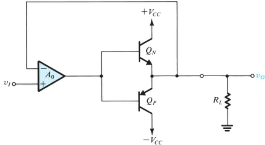
Figure x4.1 Class B circuit with an op amp connected in a negative-feedback loop to reduce crossover distortion.
