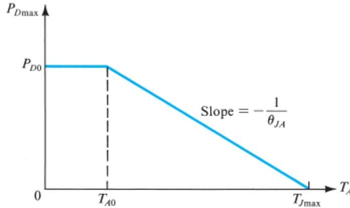
**Figure x4.7** Maximum allowable power dissipation versus ambient temperature for a BJT operated in free air. This is known as a “power-derating” curve.
