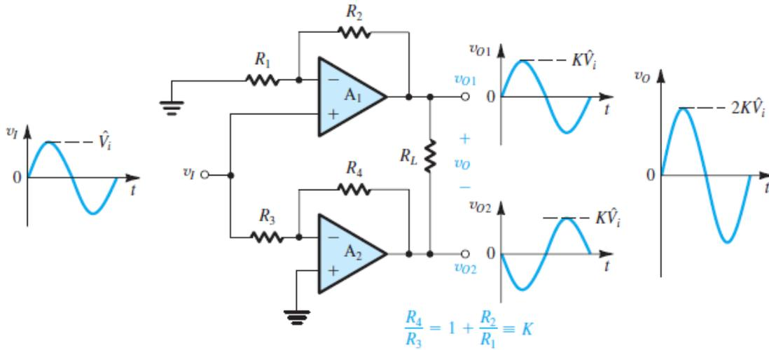
Figure x4.14 The bridge amplifier configuration.
