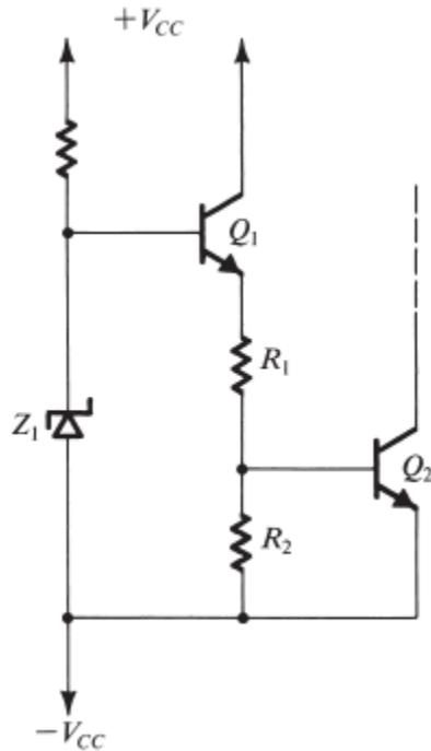
Figure x4.4 Thermal-shutdown circuit.
