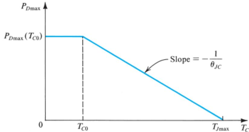
Figure x4.9 Maximum allowable power dissipation versus transistor-case temperature.
