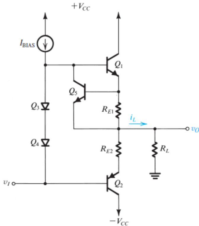
**Figure x4.3** A class AB output stage with short-circuit protection. The protection circuit shown operates in the event of an output short circuit while  $v_O$  is positive.
