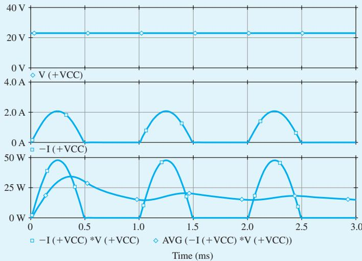
Figure B.56 The voltage (upper graph), current (middle graph), and instantaneous and average power (bottom graph) supplied by the positive voltage supply (+ $V_{CC}$ ) in the circuit of Fig. B.54.
