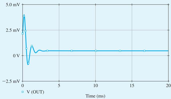
(c)  $R_{1a} = 25 \text{ k}\Omega$ , Loop Gain = 0.8
