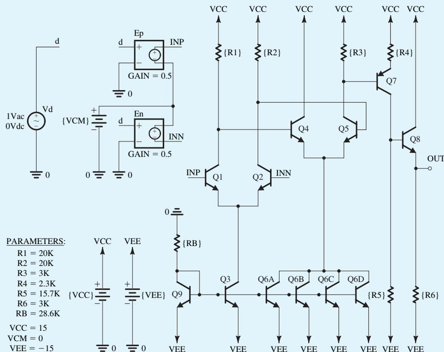
Figure B.29 Schematic capture of the op-amp circuit in Example 9.7.
