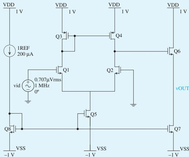
Figure B.47 Schematic capture of the two-stage CMOS op amp.
