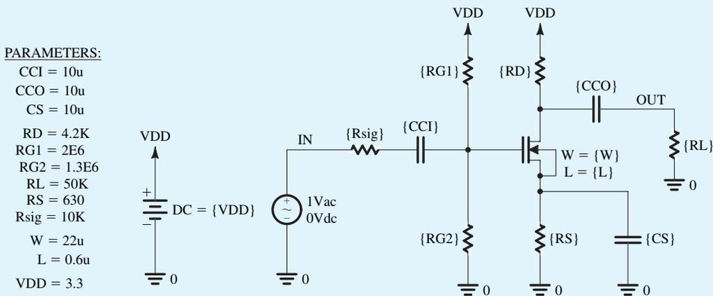
Figure B.19 Schematic capture of the CS amplifier in Example S.7.1.
