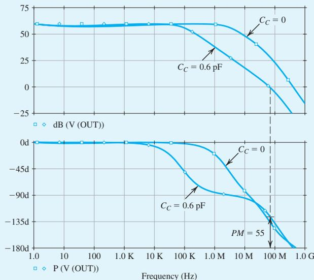
**Figure B.61** Magnitude and phase response of the op-amp circuit in Fig. B.43:  $R = 1.53 \text{ k}\Omega$ ,  $C_C = 0$  (no frequency compensation), and  $C_C = 0.6 \text{ pF}$  ( $PM = 55^\circ$ ).
