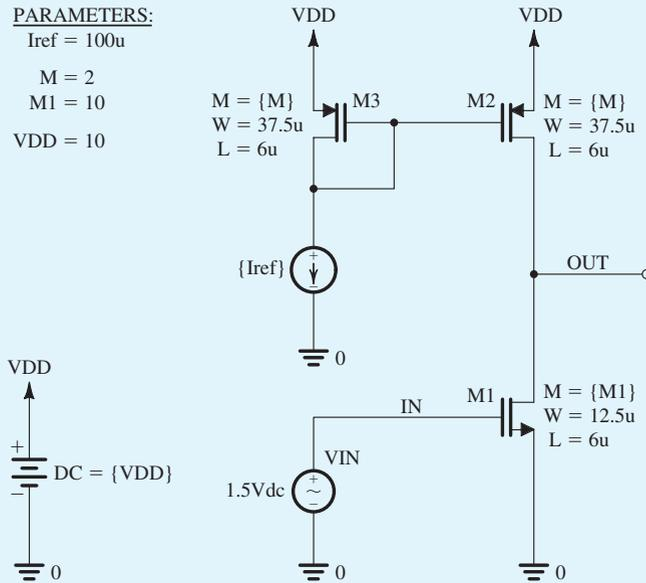
**Figure B.26** Schematic capture of the CS amplifier in Example S.8.1.
