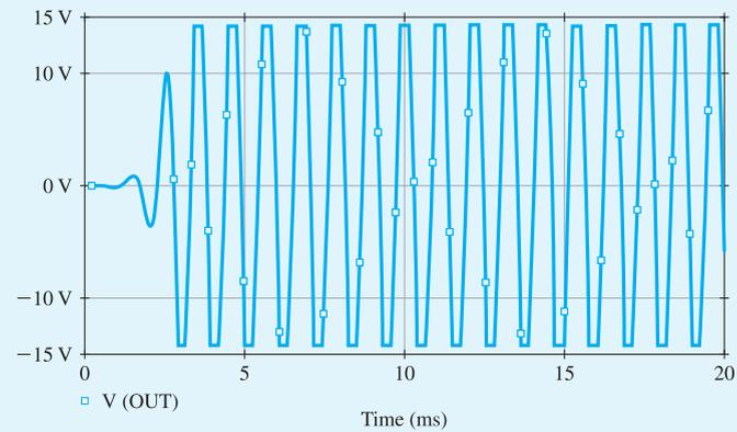
(a)  $R_{1a} = 15 \text{ k}\Omega$ , Loop Gain = 1.33
