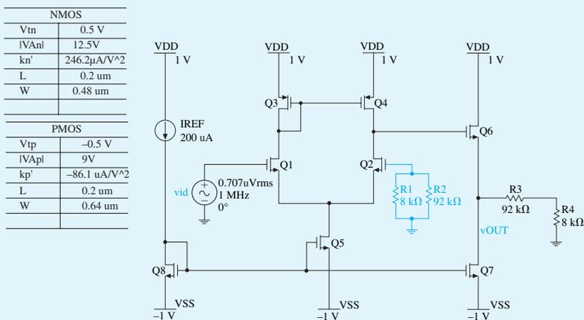
Figure B.50 Schematic capture of the A-circuit.
