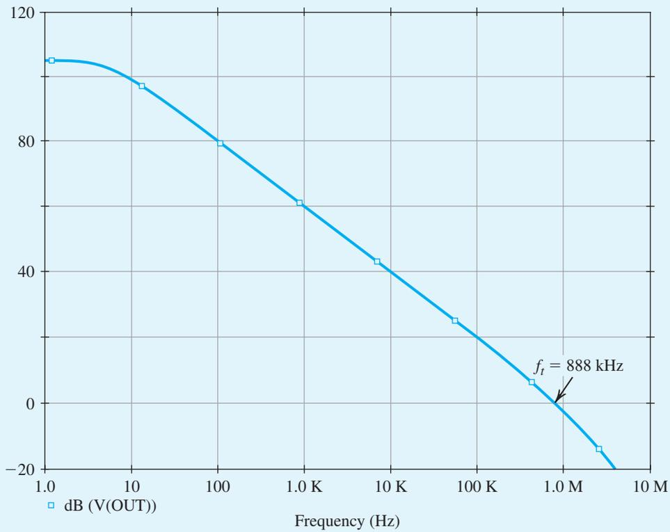
Figure B.10 Frequency response of the  $\mu$ A741 op amp in Example S.2.2.
