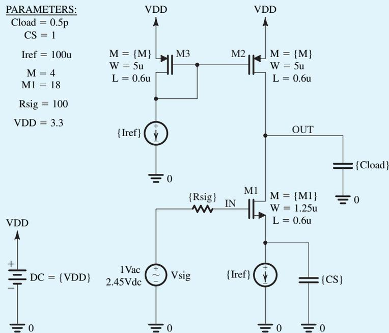
Figure B.37 Schematic capture of the CS amplifier in Example S.10.1
