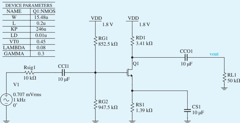
Figure B.40 Schematic capture of discrete CS amplifier.
