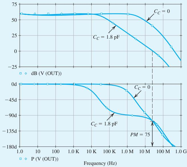
Figure B.62 Magnitude and phase response of the op-amp circuit in Fig. B.60:  $R = 1.53 \text{ k}\Omega$ ,  $C_c = 0$  (no frequency compensation), and  $C_c = 1.8 \text{ pF}$  ( $PM = 75^\circ$ ).
