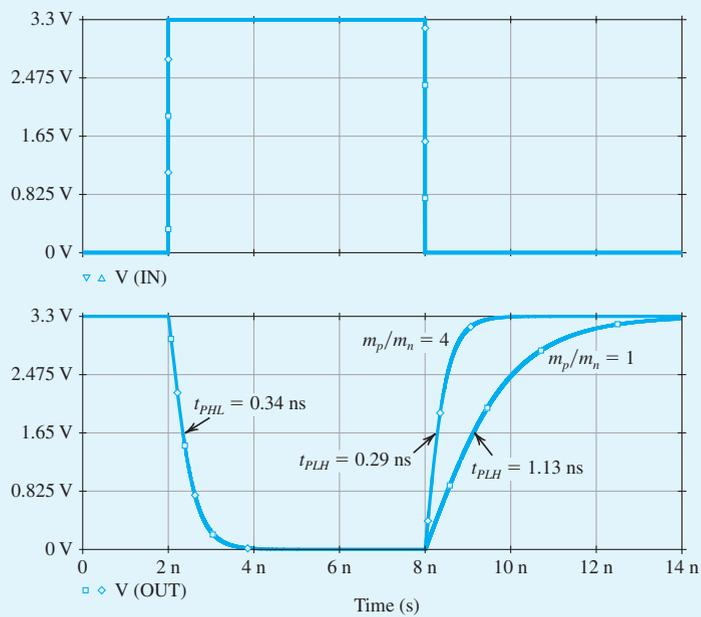
**Figure B.79** Transient response of the CMOS inverter in Example S.16.1 with  $m_p/m_n = 1$  and  $m_p/m_n = 4$ .
