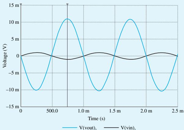
Figure B.25  $A_v$  and  $G_v$  of the CS amplifier: transient analysis.
