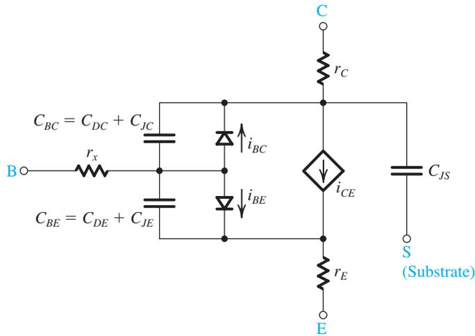
**Figure B.6** The SPICE large-signal model for an *nnp* BJT.
