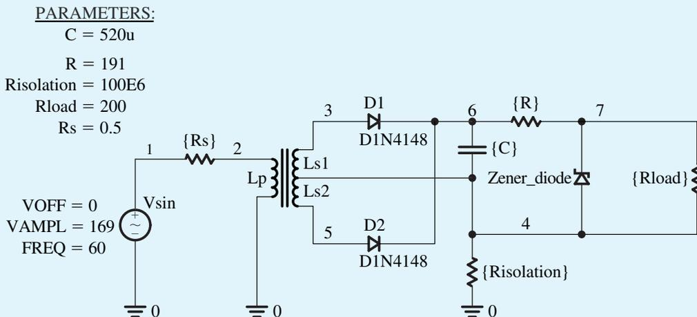
Figure B.13 Schematic capture of the 5-V dc power supply in Example S.4.1.
