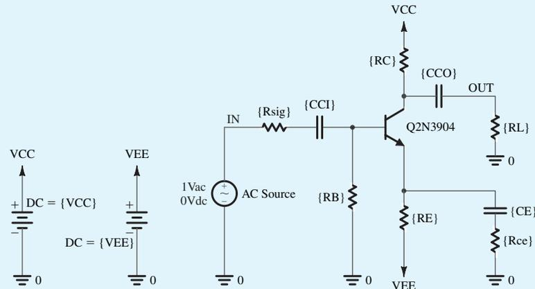
**Figure B.21** Schematic capture of the CE amplifier in Example S.7.2.
