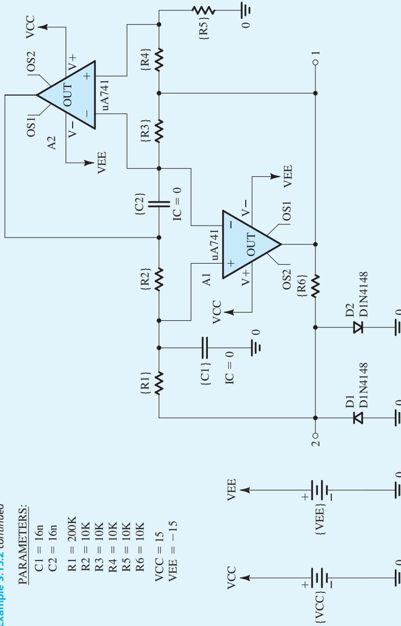
**Figure B.74** Example S.17.2: Schematic capture of an active-filter-tuned oscillator for which the  $Q$  of the filter is adjustable by changing  $R_1$ .
