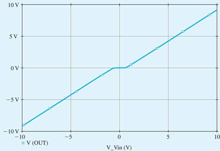
**Figure B.58** Transfer characteristic of the class B output stage of Fig. B.54.
