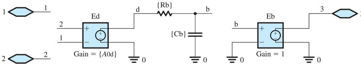
**Figure B.1** A linear macromodel used to model the finite gain and bandwidth of an internally compensated op amp.
