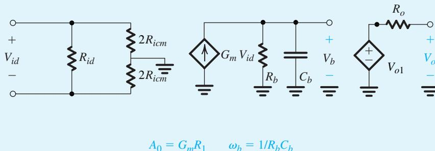
**Figure B.68** One-pole equivalent-circuit macromodel of an op amp operated within its linear region.
