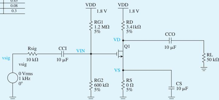
Figure B.23 Capture schematic of the CS amplifier.
