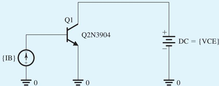
**Figure B.17** The SPICE test bench used to demonstrate the dependence of  $\beta_{dc}$  on the collector bias current  $I_C$  for the Q2N3904 discrete BJT (Example S.6.1).
