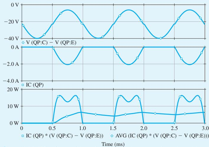
**Figure B.57** Waveforms of the voltage across, the current through, and the power dissipated in the  $pnp$  transistor  $Q_p$  of the output stage shown in Fig. B.54.
