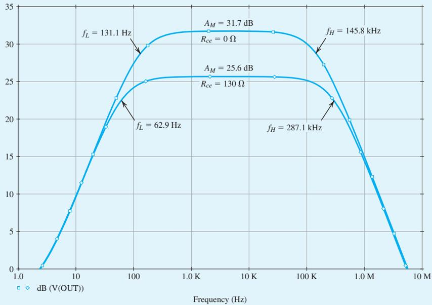
**Figure B.22** Frequency response of the CE amplifier in Example S.7.2 with  $R_{ce} = 0$  and  $R_{ce} = 130 \Omega$ .
