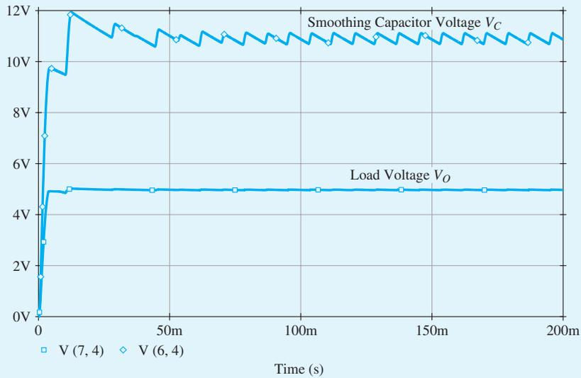
**Figure B.14** The voltage  $v_c$  across the smoothing capacitor  $C$  and the voltage  $v_o$  across the load resistor  $R_{\text{load}} = 200 \Omega$  in the 5-V power supply of Example S.4.1.
