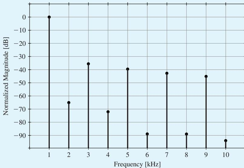
Figure B.59 Fourier-series components of the output waveform of the class B output stage in Fig. B.54.
