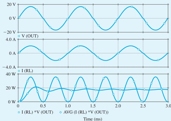
Figure B.55 Several waveforms associated with the class B output stage (shown in Fig. B.54) when excited by a 17.9-V, 1-kHz sinusoidal signal. The upper graph displays the voltage across the load resistance, the middle graph displays the load current, and the lower graph displays the instantaneous and average power dissipated by the load.
