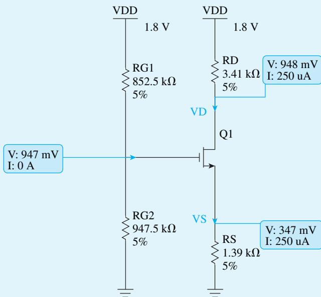
Figure B.24 DC bias-point analysis of the CS amplifier.
