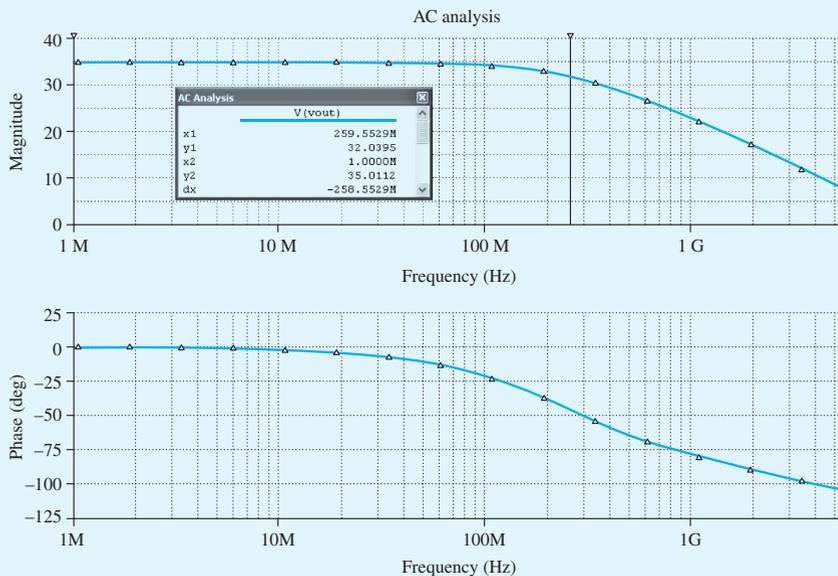
Figure B.49 Frequency response of the two-stage CMOS op-amp amplifier.
