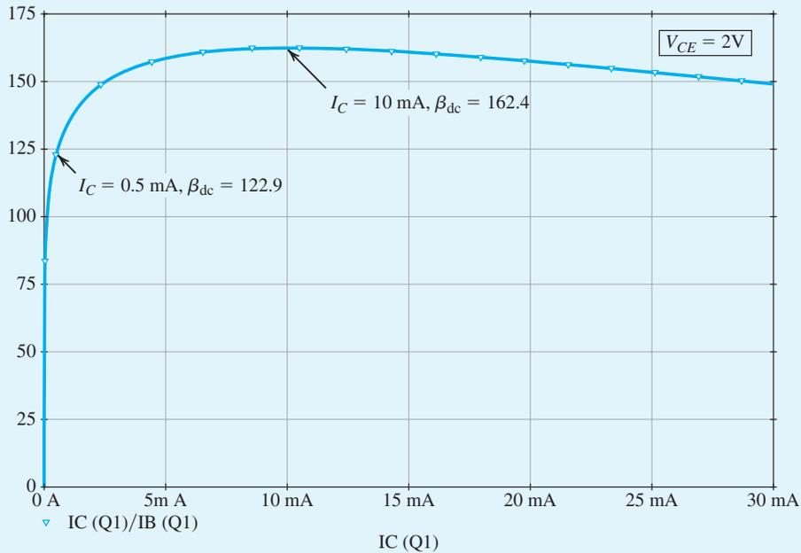
**Figure B.18** Dependence of  $\beta_{dc}$  on  $I_C$  (at  $V_{CE} = 2\text{ V}$ ) in the Q2N3904 discrete BJT (Example S.6.1).
