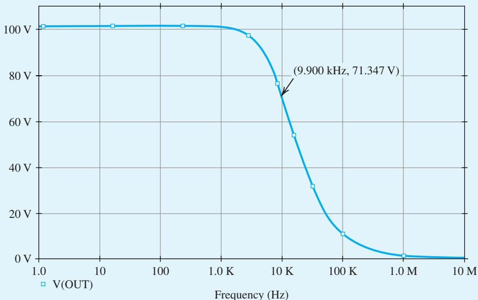
Figure B.7 Frequency response of the closed-loop amplifier in Example S.2.1.
