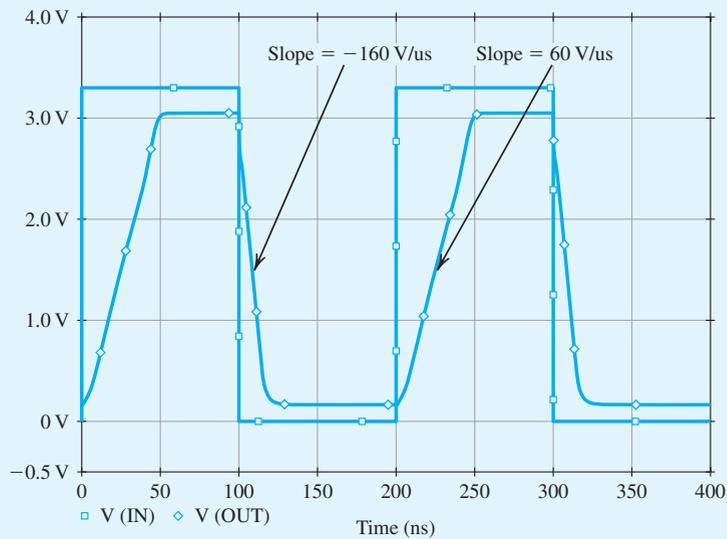
**Figure B.65** Large-signal step response (for a 3.3-V step-input) of the op-amp circuit in Fig. B.60 connected in a unity-gain configuration. The slope of the rising and falling edges of the output waveform correspond to the slew rate of the op amp.
