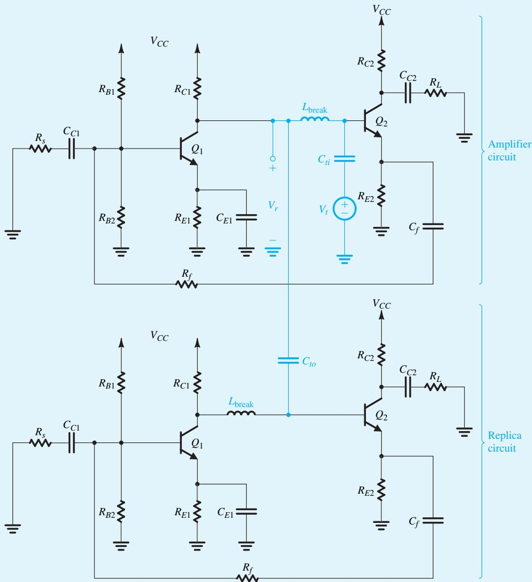
**Figure B.45** Circuit for simulating the loop gain of the feedback amplifier circuit in Fig. B.43 using the replica-circuit method.
