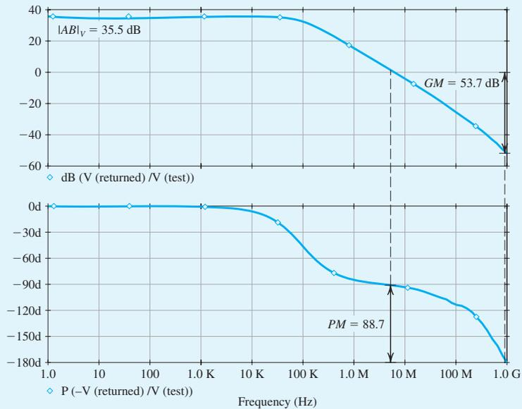
**Figure B.46** (a) Magnitude and (b) phase of the loop gain  $A\beta$  of the feedback amplifier circuit in Fig. B.43.
