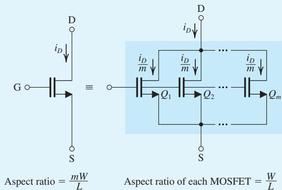
**Figure B.27** Transistor equivalency.
