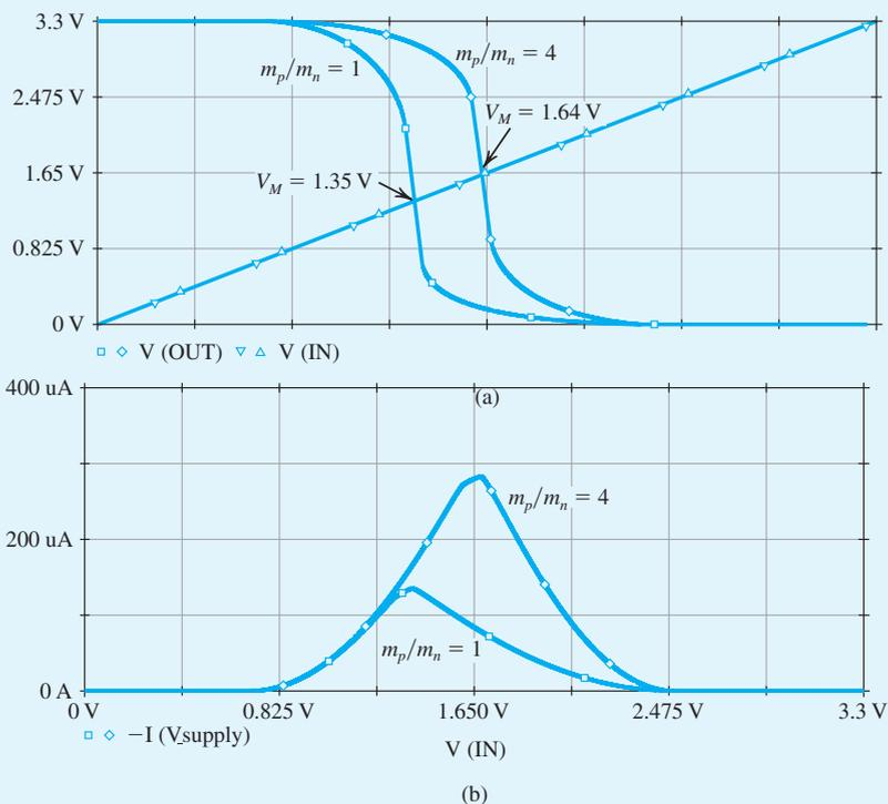
Figure B.78 (a) Output voltage and (b) supply current versus input voltage for the CMOS inverter in Example S.16.1 with  $m_p/m_n = 1$  and  $m_p/m_n = 4$ .
