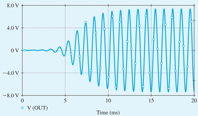
(b)  $R_{1a} = 18 \text{ k}\Omega$ , Loop Gain = 1.1
