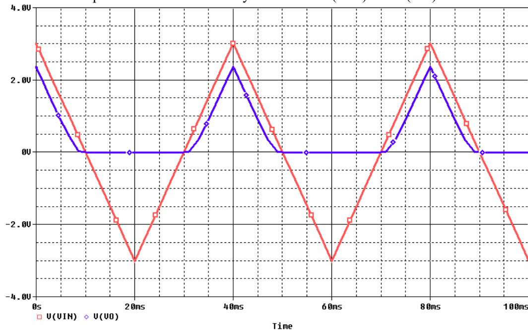
3. Calculate the average of  $V_{(VO)}$  by using the trace expression  $\text{YatLastX}(\text{AVG}(V(VO)))$  (*this expression is valid only in PSpice. Enter this expression by selecting Trace->Evaluate Measurement*). It is 504.6 mV
