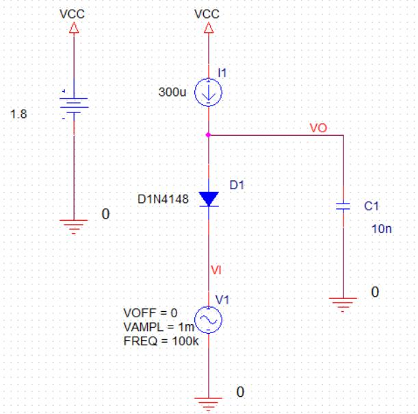
2. Run the netlist and perform the transient analysis. Plot  $V(VI)$  and  $V(VO)$ . For -45 degree phase shift the waveform should shift by 1.25 us. It happens when  $I=160\mu A$ .
