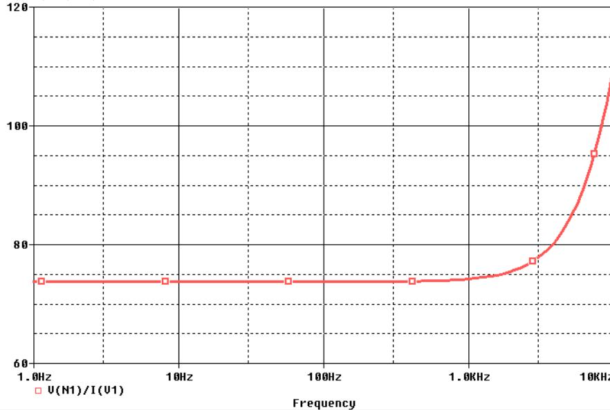
13. The input impedance is  $74 \Omega$ .
