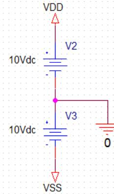
8. Run the netlist and perform an operating point analysis. The node voltages are
