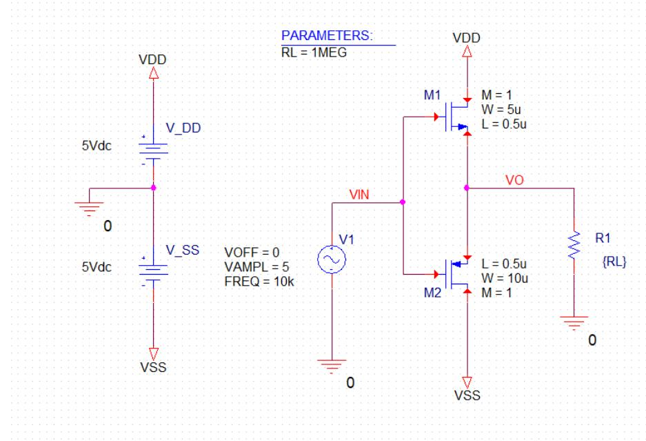
2. Run the netlist and perform a transient analysis. Plot  $V(VIN)$  and  $V(VO)$  as shown below.
