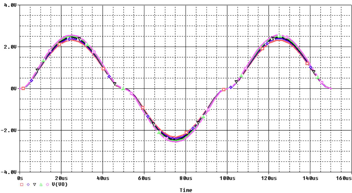
6. The output voltage is half of the input voltage when  $RL = 650 \Omega$ .
