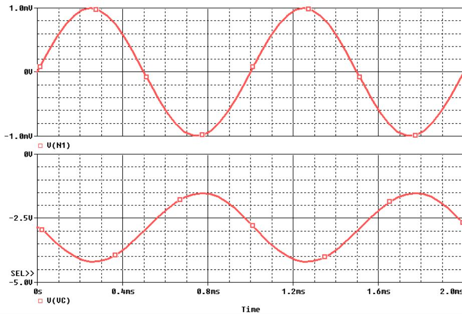
11. The gain from this simulation is 1335 V/V.
