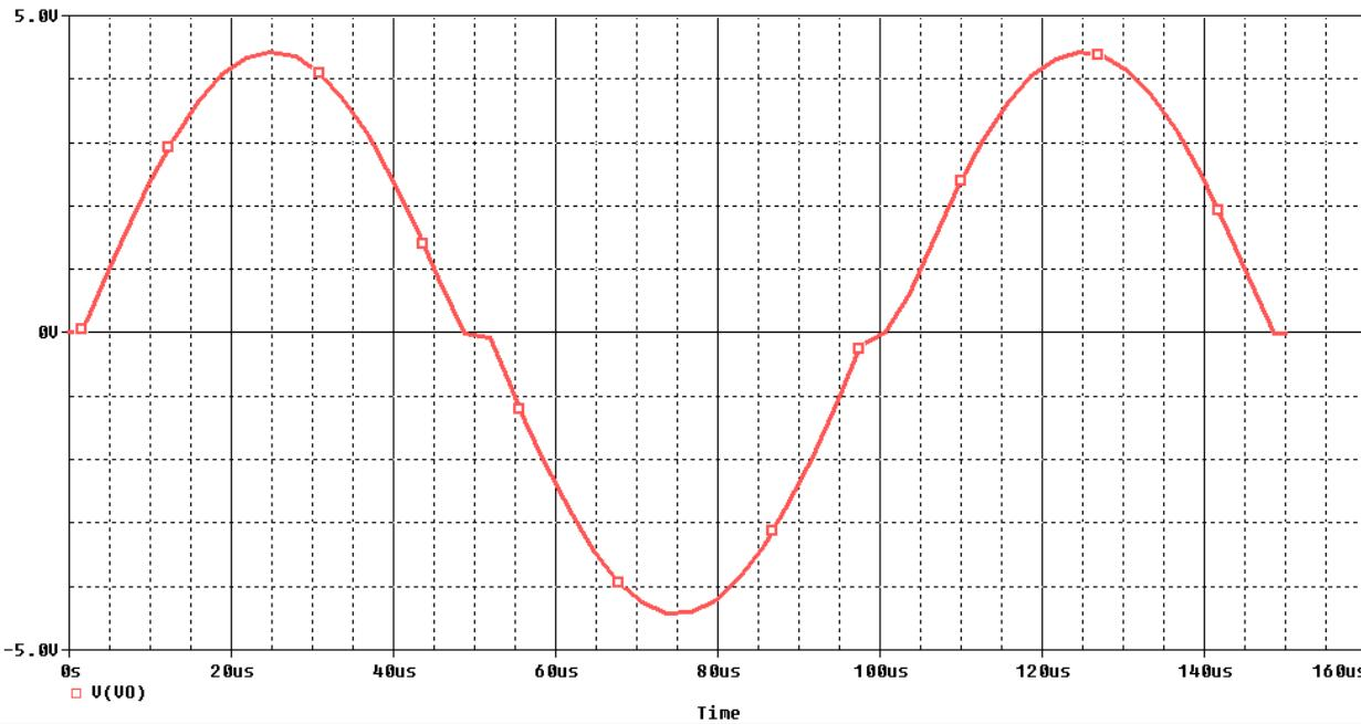
3. The output  $V(VO)$  swings from 4.42 V to -4.41 V.
